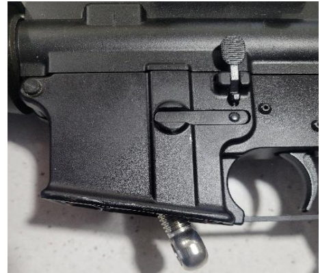
Figure 8: Locking Magazine inserted into the rifle's magazine well and the Pivot Locking Arm is shown pivoted into the rifle's barrel.
