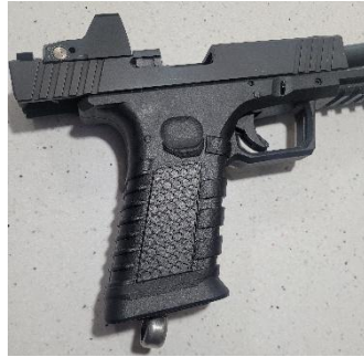
Figure 13. The Locking Magazine inserted and locked into the barrel by the pivoting arm.
