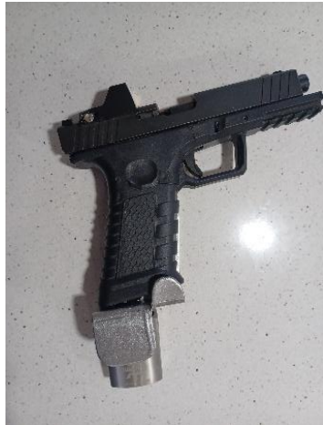
Figure 15. The Locking Magazine locked on the Locking Magazine Base with the pad lock.
