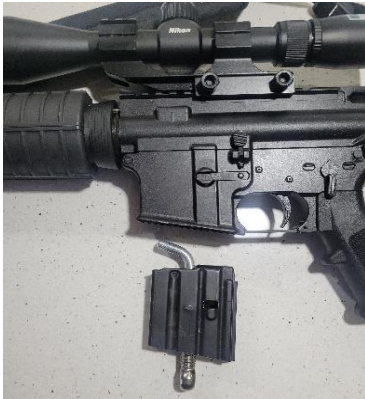
Figure 6: Locking Magazine in position to be inserted into the rifle's magazine well.
