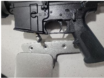
Figure 9: Locking Magazine is in position to be inserted into the Locking Magazine Base
